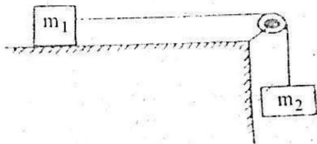
In the diagram above, the hanging mass  $m$  is adjusted until  $m$  is on the verge of sliding. The
